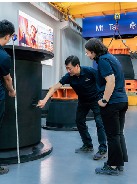
Measuring fenders at the Qingdao test facility.
