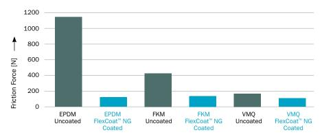
In endurance and assembly force tests, FlexCoat™ NG gave superior performance results.
