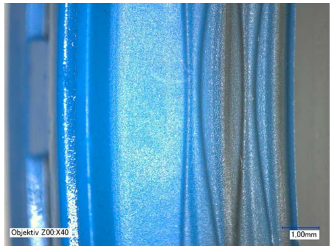
Inspection of seal after endurance test shows no signs of wear.
